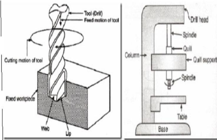
Working principle: The rotating edge of the drill exerts a large force on the workpiece and the hole is generated. The removal of metal in a drilling operation is by shearing and extrusion.
